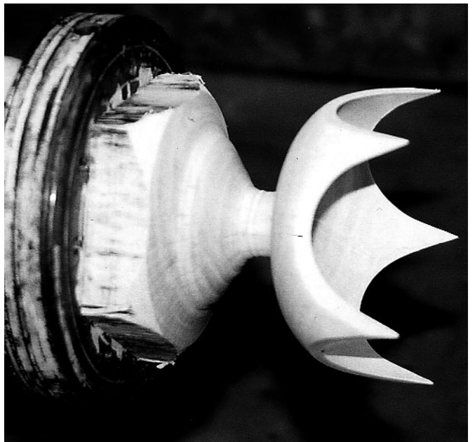
PHOTO 4: Outside finished and ready for parting off. All photos by the author.
