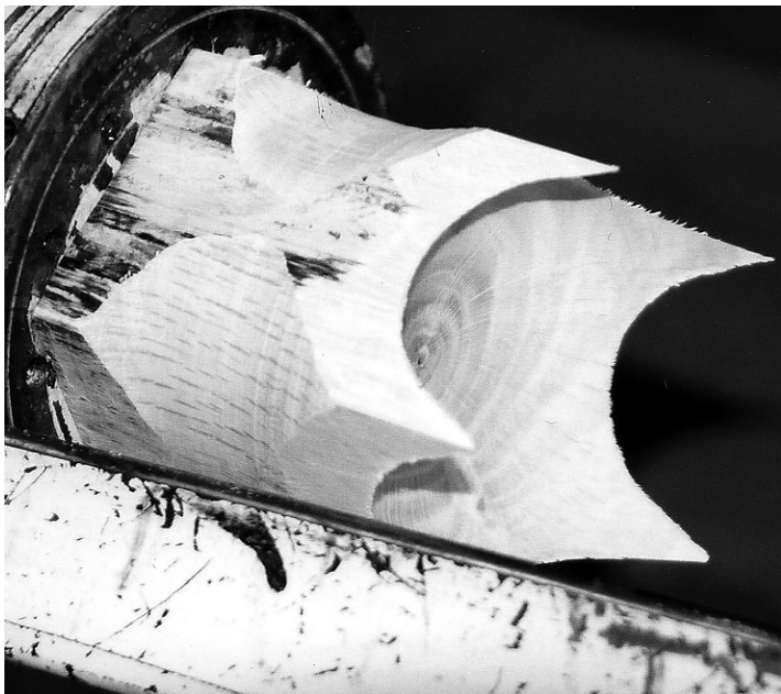
PHOTO 3: The inside finished and sanded and the first outside cuts made. Note: wall thickness is about 1/2-in. at this point.
