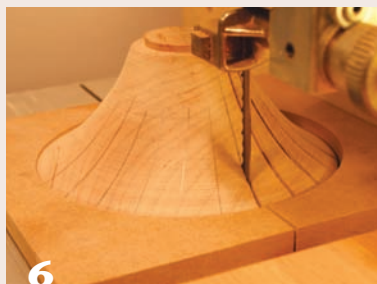
6 With the bowl held in a jig, cut along each radial line. Note the stop clamped onto the bandsaw table, behind the jig.
