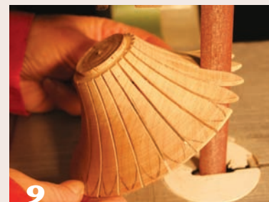
9 Sand and shape the petals using a belt sander.
