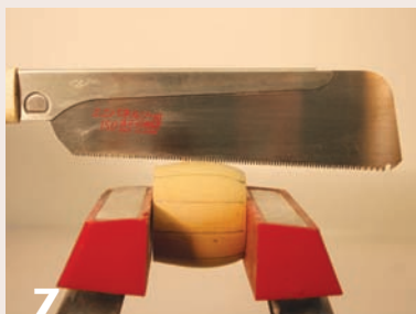
7 For safety, cut the twelve radial lines in the smallest bowl using a handsaw.
