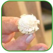
and use the tailstock to center the piece. Round the piece out and remove the bark. Remove the tailstock. Apply the heel-end of a skew to the free-end of the stick to peel back very thin layers of
